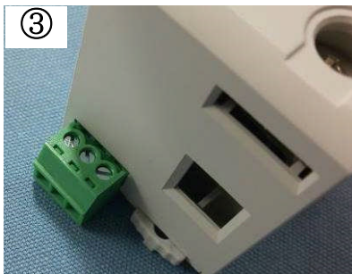
Fig.9-3 Connection of terminal block
